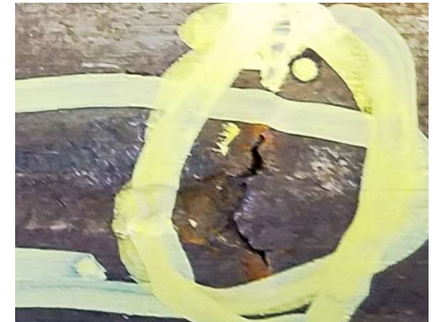
Photo after sample failure in fatigue machine
