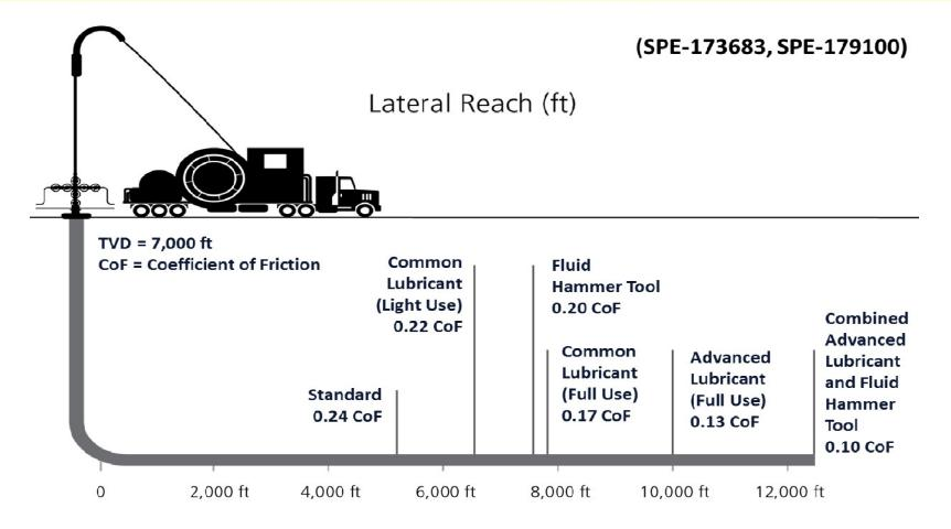
Note: Sample analysis 2" CT in 5½" horizontal well. Ability to transfer 500 lbf available weight on bit for each condition listed above.
