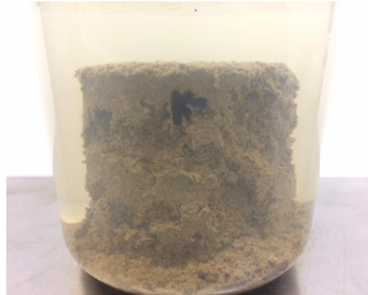
Unstable soil after soaking
