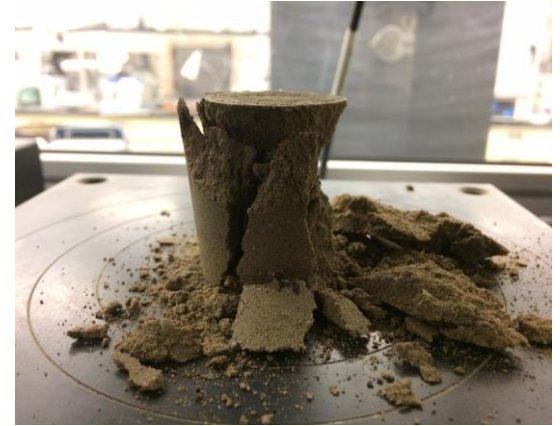
Stabilized soil after crushing
