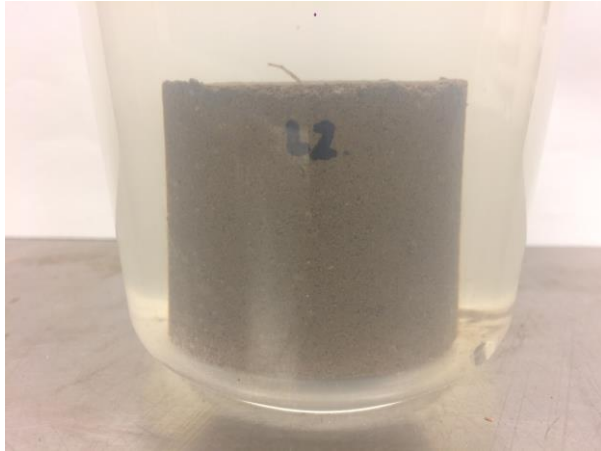
Stabilized soil after soaking
