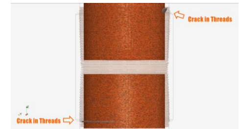
Parted & Cracked Connections
