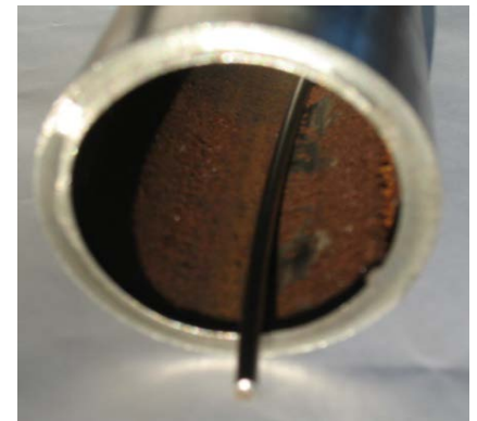
1/8" TeleCoil conductor in 2" CT
